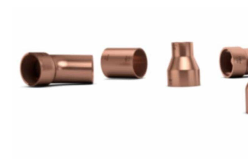
Developed in conjunction with Wieland K65 high strength copper alloy fittings enable simple, safe and economical installation of high pressure refrigeration applications up to 130 bar. K65 fittings are particularly suited for use with CO<sub>2</sub> (R-744) in transcritical applications.
