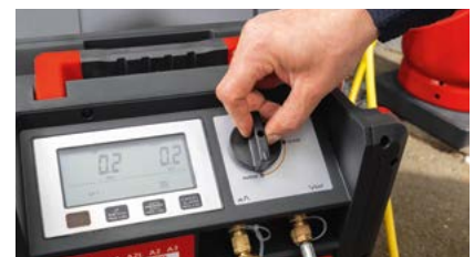
Purge function for complete draining of the recovery unit
