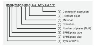
A BPHE should in principle always be denominated as shown in the figure. The different groups (1) to (8) are explained to the left.
