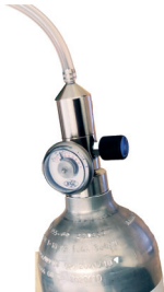
Once the required gas cylinder is available, screw the pressure reducer onto the cylinder, keeping the valve closed so that no gas is released.
